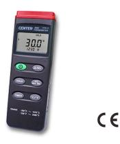
**Specifications** Details K type: -200~1370â□□ ; -328~2498â□□ Range Resolution 0.1â[]; 0.1â[]] ±0.3%+1â□□, ±0.3%+1.8â□□ Accuracy **Operating Temperature** 0â□□~50â□□ (<80%RH) Storage Temperature -20â[]]~60â[]] (<70%RH) Battery 9V battery Dimensions 184x64x30 mm Weight Approx.210g
