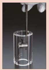
The handle extension enables measurement deep within a hole.
