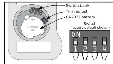
To change the resolution from 0.1°C (factory default) to 1°C push the switch away from the batteries.
