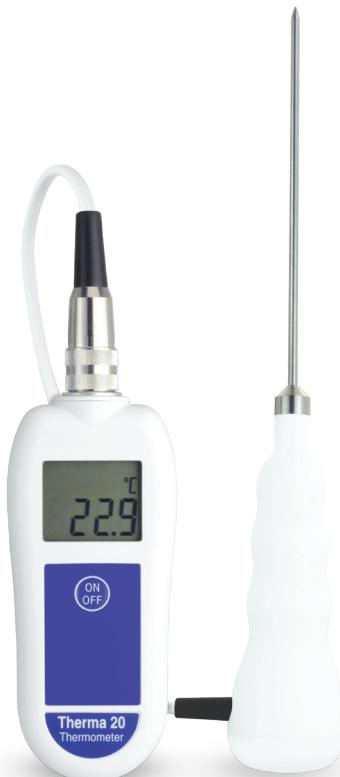
**INSTRUMENT OPERATION** - Where applicable (Therma 20 and Therma 22) connect a probe via the socket located at the top of the instrument, screw in the collar of the plug, finger tight, to ensure a secure connection (do not over tighten). Switch the instrument on and apply the tip of the probe to the substance or medium to be measured. The instrument reading may take a few seconds to stabilise, depending on the nature of the measurement and sensitivity of the probe.
