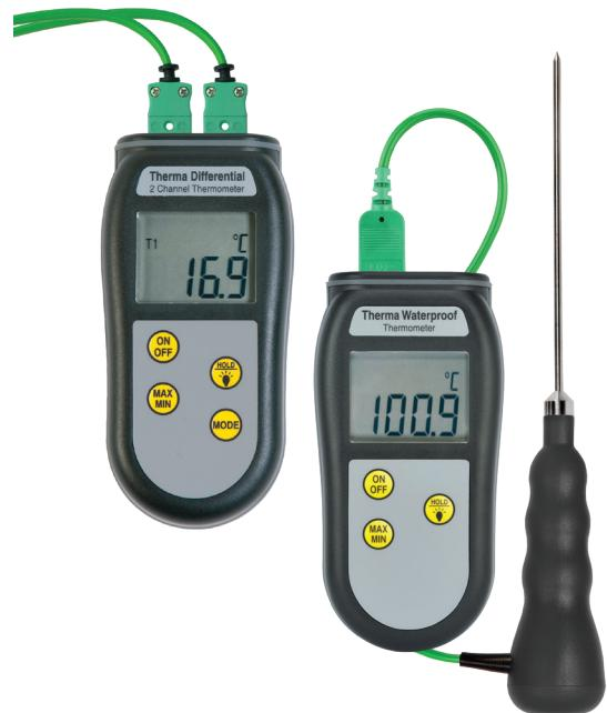
**INSTRUMENT OPERATION** - Connect probes via the socket(s) located at the top of the instrument. (The Therma Waterproof and Therma Differential use a miniature type K thermocouple connector(s). Switch the instrument on and apply the tip of the probe to the substance or medium to be measured. The instrument reading may take a few seconds to stabilise, depending on the nature of the measurement and sensitivity of the probe.
