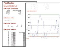
A simple gage interface to retrieve data in a manner similar to USB flash drives or cameras. No software to install or internet connection required. Measurement data can be printed quickly from a formatted HTML report or exported in .csv format for further analysis in spreadsheets.
