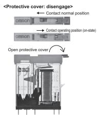
Keep the protective cover open when using the latching lever. Move until the latching lever clicks to the ON position (ON state). After use latching lever, in order to prevent malfunction, return the switch to contact normal position (OFF state), and make sure the protective cover is firmly closed.
