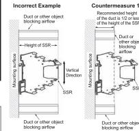
Do not enclose the SSR in a duct of the same height It will interfere with the heat dissipation of SSR.
