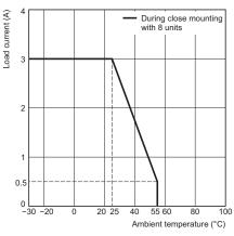
\* When eight or more are installed, install with 10 mm space between each. For details, please refer to *Mounting* on page 28.
