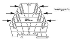
• When removing the PLC interface, place a finger at the place below and pull it out.
