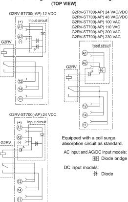
**Terminal Arrangement/Internal Connection Diagram**
