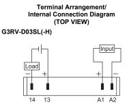
**Note:** The load can be connected to either the positive or negative terminals.
