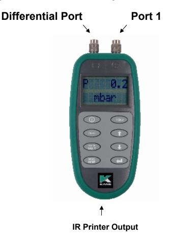
Always use the top right hand port (Port 1) for taking single channel measurements (pressure or vacuum). Only use the left hand port for differential measurements.
