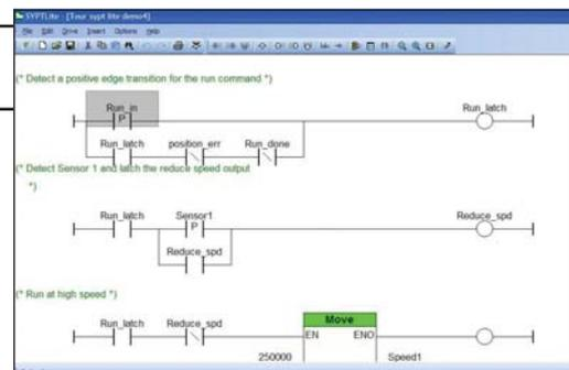
Replace nano and micro PLCs by using the LogicStick and SyPTLite giving ladder and function block programming for timers, counters, latches, etc – to get the most from SK's intelligence option.
